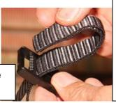
**NOTE**: There is a top and bottom to a buckle. Notice that the ribs on the center bar of the buckle are on top. When properly assembled the strap and buckle will **not** slip and loosen easily.
